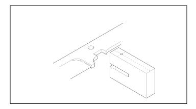
Fit the guard to the blade making sure it fits tightly in place.
