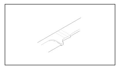
Drill an oversize hole on the centre line leaving at least 5mm from the top of the blade to the top of the hole.
