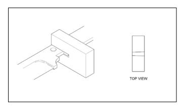
Once the slot is a nice fit on the blade it is time to work on the thickness of the guard.
