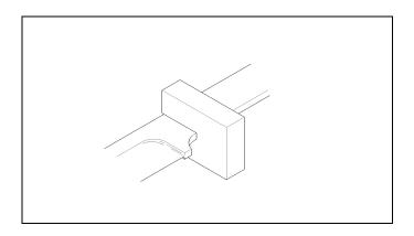
Mark a centre line down the length of the side of the guard where the pin hole is to be drilled. Measure the distance from the top of the blade to the centre of the brass rod in the blade and add the amount of protrusion that was previously measured. Carry this measurement over to the guard and mark where the pin will be. Centre punch this mark.
