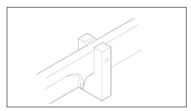
The top of the guard can now be ground flush with the blade.
